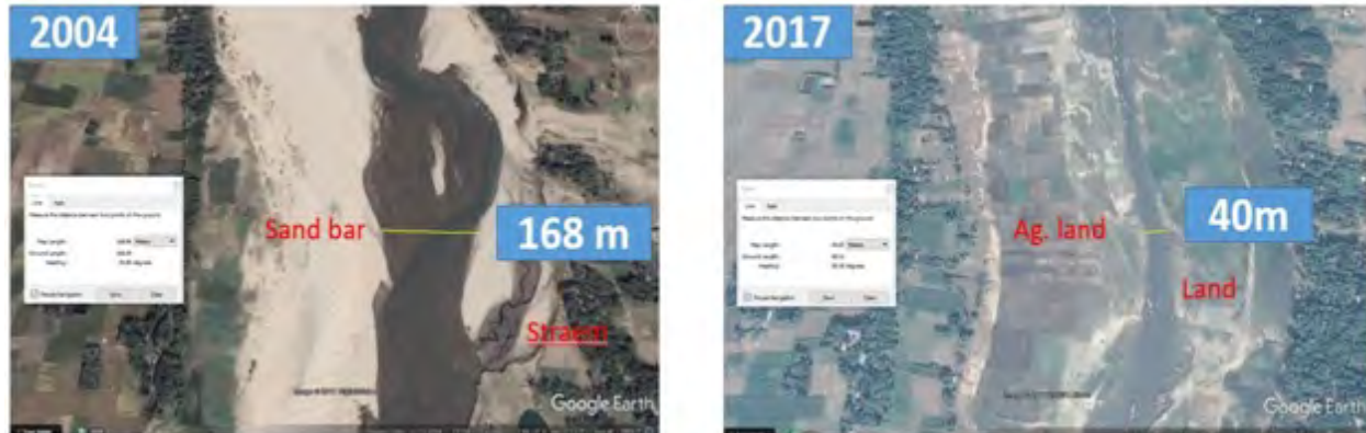
Figure 5: Aerial image showing the changes in width of the Jadukata River between 2004 and 2017. Both of these Goggle images were taken in December. The changes in river morphology and landuse are visible in the images. The sandbars in the river (left panel) are converted to agricultural land (right panel), reducing the carrying capacity of the river.
